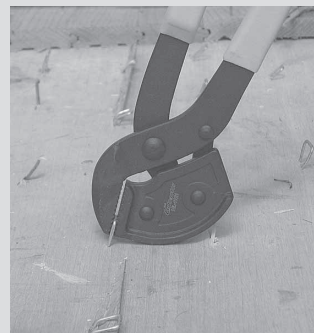
Nose on the Extractor lets you grip the complete fastener and roll it out without bending it.
