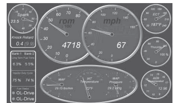
AutoTap Diagnostic Scanner lets you create a virtual dashboard of function monitors on a PDA or laptop computer.
