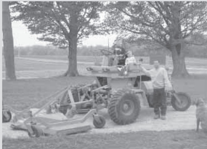
Jason Becker makes short work of cutting his large yard, thanks to his 10-ft. mower built out of an Owatonna swather.
