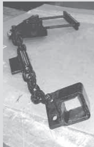
Nebgen's Deere hitch stabilizers are modeled after equipment found on Allis Chalmers' tractors.
