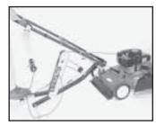
bagger and attaches to the mower handle with four adjustable clamps. Once attached to the mower, the cord is never pulled by hand. To start the mower you simply step on a pedal.
