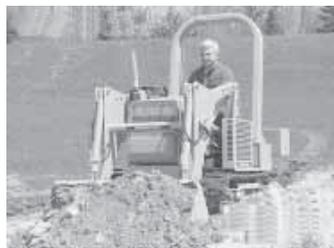
dozing, hauling, and earthmoving that's available in five models ranging from 10 to 28 hp. The 10 hp model is small enough to fit in the back of a pickup. More than 30 different attachments are available including a loader, front and rear hitch, six-way blade, backhoe, auxiliary hydraulic circuit, PTO-operated auger, scarifier/ripper, log splitter, log fork, post-hole auger, plow, etc.
