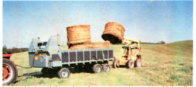
By removing the roof, sides and rear door you can use the wagon as a 6-bale trailer. Put a beater at the rear and add "slop" gates and you can use it as a manure spreader.
