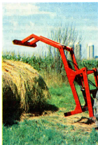
One hydraulic cylinder pinches the bale grabbing arms together and the other lifts the bale upward once it's been grabbed.
