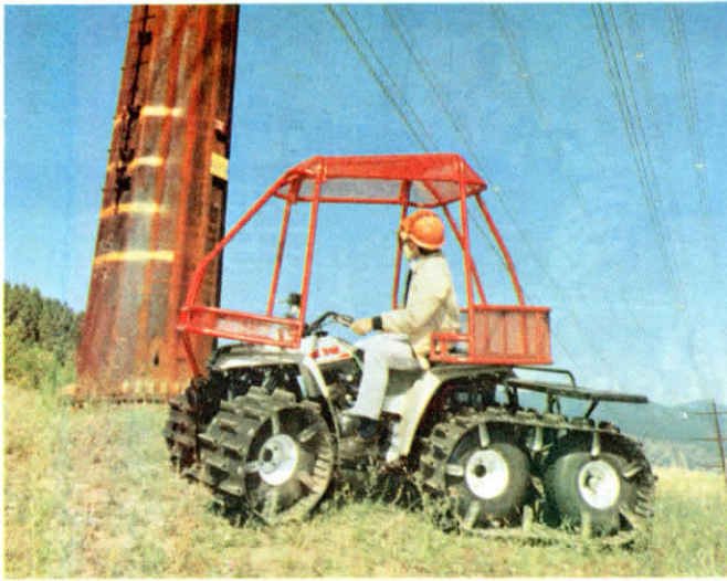
Big Foot tracks include a second rear axle and an additional set of wheels.
