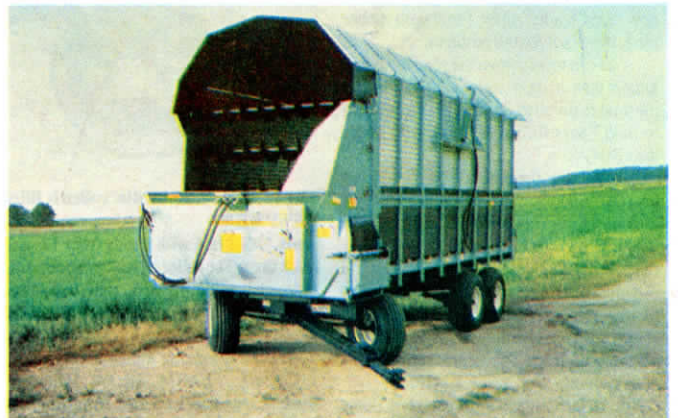
With roof and sides in place wagon serves as a forage wagon (front or rear unload).
