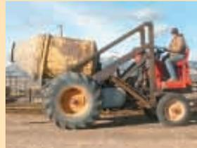
Self-Propelled Concrete Mixer
