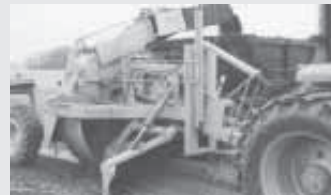
The pto-operated ditcher consists of an 8-ft. dia. steel wheel fitted with 8 bolt-on digger buckets. It also has a laser grade control system.
