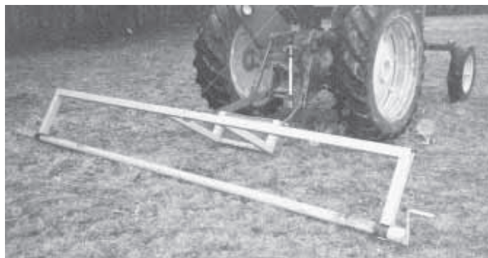
Tractor-mounted roller makes it easy to roll up wide sheets of plastic covering crop.
