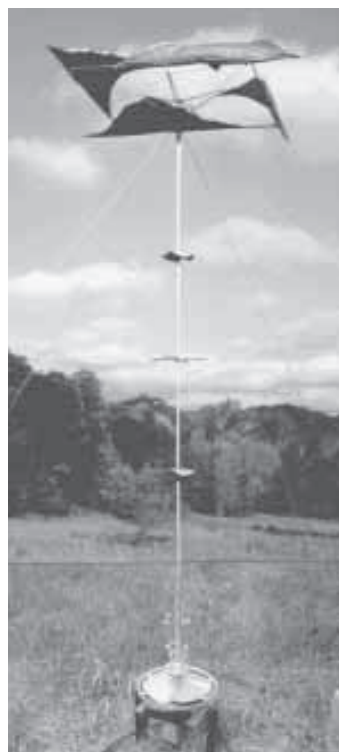
Easy-to-use portable windmill uses collapsible sails instead of blades to generate mechanical power.
