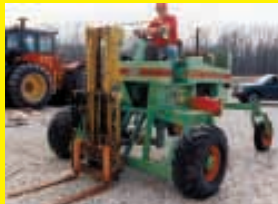
Swather Fitted With Forklift (Page 18)
