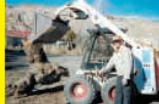
Skid Steer Controlled From Outside Cab (Page 43)
