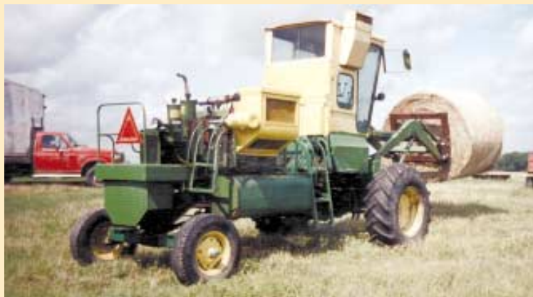
To offset the weight of loader up front, Snellings added a big steel box on back that's full of concrete and strap iron.
