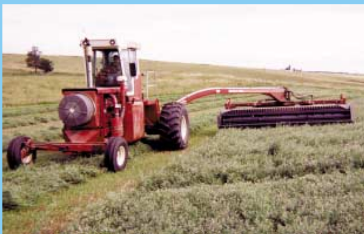
Crick uses his "combine tractor" mainly to pull a windrower. The tractor has a wide wheelbase, allowing it to straddle any size windrow.
