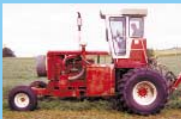
He turned the cab around to face what had been the rear of the combine.
