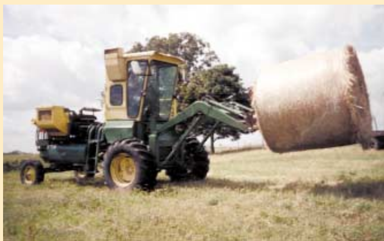
"It works great for hauling round bales," says Gene Snellings, who converted a pair of Deere 55 combines into a loader tractor.
