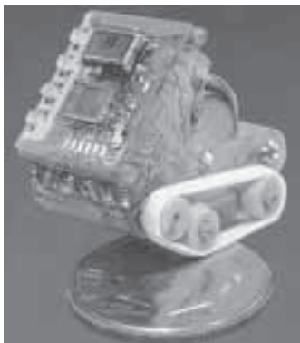
The world's smallest robot was built at Scandia National Laboratories using a number of parts supplied by Small Parts Inc. The plan is to fit the robots with temperature sensors, radios, microphones, and other devices for gathering information in the event of chemical spills.
