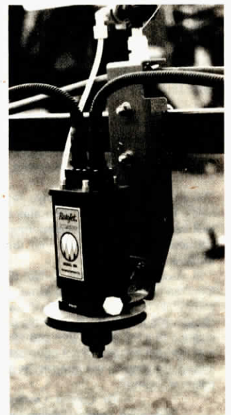
All electric components are enclosed on the rugged new spray head.
