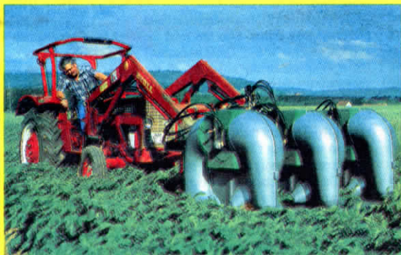
Bug-Sucking Vacuum - Hydraulic-powered blower-vacuum knocks insects off plants with a blast of air and then sucks them up for disposal. (See p. 23)
