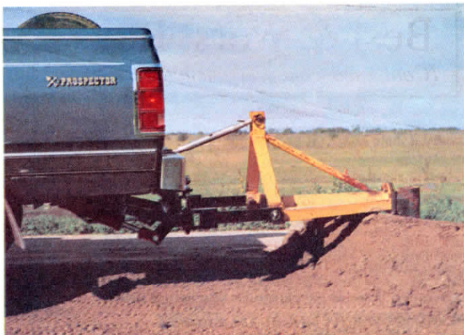
Hitch bolts to bumper and main frame of pickup. Hydraulic pump mounts between the twin lifting cylinders.
