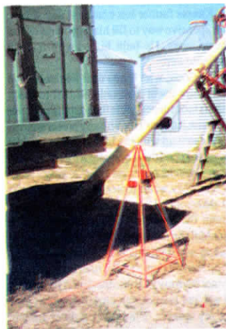
When back of truck hits spring-loaded aerial on top of 4-legged stand, it trips a switch which activates a red "stop" light.
