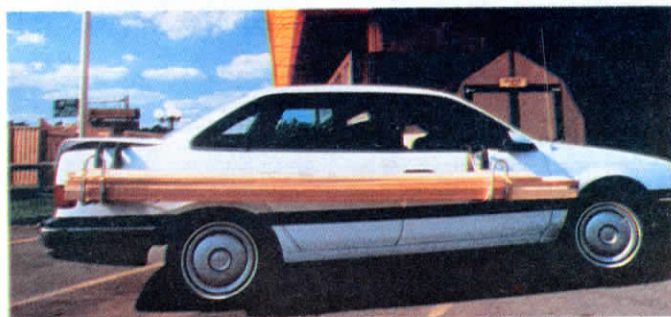
Hooks fit over edge of trunk and car door (with window open). They'll also hang from a pickup door and box.
