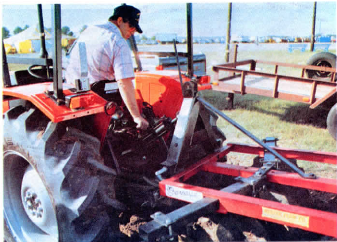
Hitch consists of two V-shaped steel frames, one that mounts on tractor 3-pt. and the other on implement.
