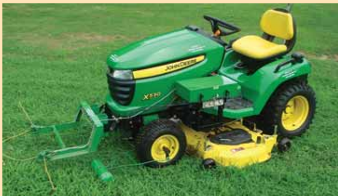
Riding mower has 2 coil sensors mounted on front, one on each side (above). Sensors follow underground wire and send information to an electronic box, which in turn operates a motor that's used to control mower's steering system.
