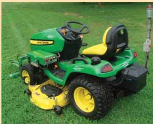
Riding mower has 2 coil sensors mounted on front, one on each side (above). Sensors follow underground wire and send information to an electronic box, which in turn operates a motor that's used to control mower's steering system.
