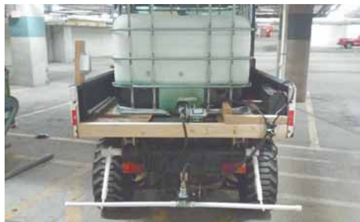
Michael Gresch added this pvc spray boom on back of a Bobcat utility vehicle. It's used to spray waste brine containing up to 10 percent salt.
