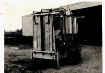
Chemical spray from unit's 28 nozzles is recycled after it drains off animal.
