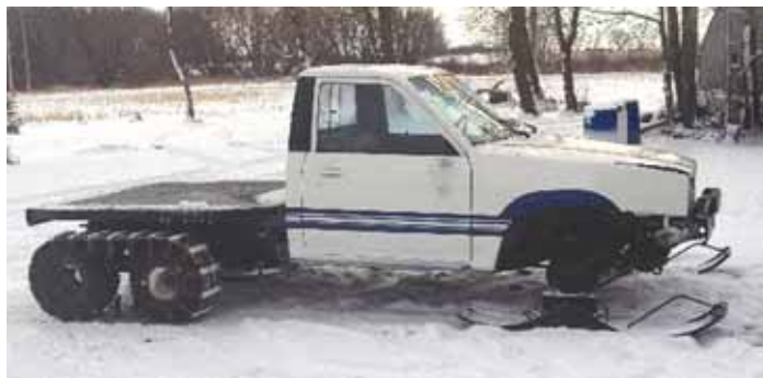
Josh Eddy converted a 1986 Mazda 2-WD pickup into this big "snowmobile" that has 4-ft. long curved metal skis on front and 4-ft. long cleated rubber tracks on back. He started by cutting 2 ft. out of the pickup's frame and then welding it back together.
