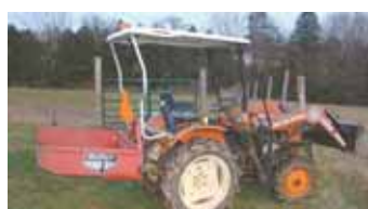
Steve Browning made a shade canopy for his 18 hp Kubota loader tractor from the top of a junked golf cart.
