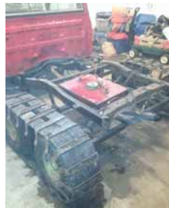
Josh Eddy converted a 1986 Mazda 2-WD pickup into this big "snowmobile" that has 4-ft. long curved metal skis on front and 4-ft. long cleated rubber tracks on back. He started by cutting 2 ft. out of the pickup's frame and then welding it back together.
