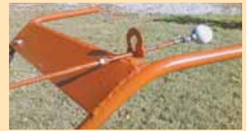
A clutch wheel with a golf ball handle is used to tighten the belts. Cutter wheel was made by bolting 12 Rayco stump grinder teeth onto a 48-tooth chain sprocket.
