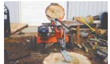
"Stump anchor" consists of piece of iron with a ball hitch bolted to one end. It bolts down to stump and sets flush with its surface.
