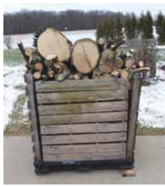
Strahle uses his home-built firewood pallets to haul and store split wood. Pallet is shown setting on 2 by 6's on concrete to keep it from freezing to the ground.
