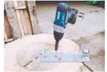
"Stump anchor" consists of piece of iron with a ball hitch bolted to one end. It bolts down to stump and sets flush with its surface.
