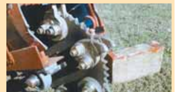
A clutch wheel with a golf ball handle is used to tighten the belts. Cutter wheel was made by bolting 12 Rayco stump grinder teeth onto a 48-tooth chain sprocket.
