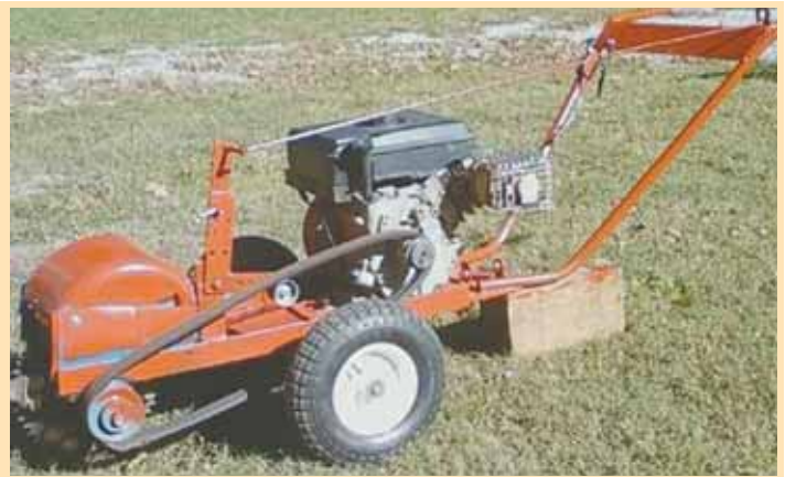
Michael Reedy's home-built stump grinder is powered by a 9 hp side shaft motor that belt-drives a cutter wheel on front.
