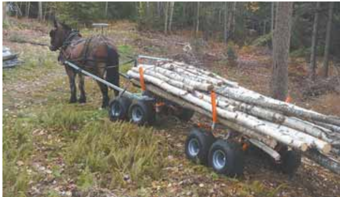
Horse-drawn log wagon is fitted with 8 bogie wheels, allowing it to carry a lot of wood over rough ground.
