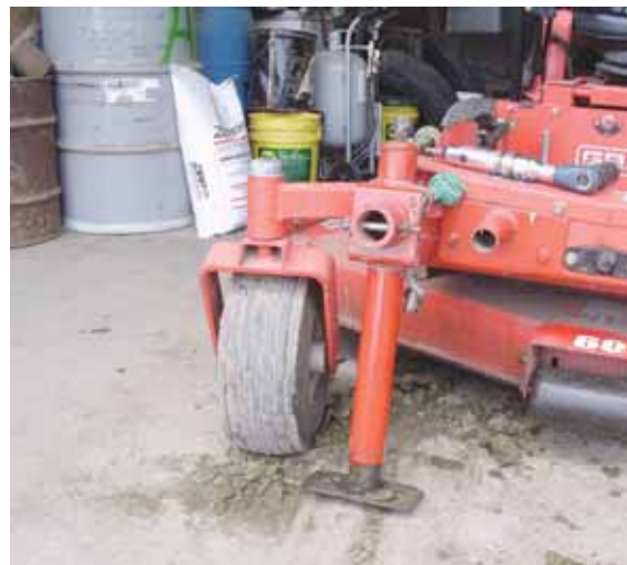
John Lubinski needed a better way to lift his Graveley zero turn riding mower for service work, so he converted a big hand-cranked lift jack off a pull-type stalk chopper. Jack pins to short piece of pipe on front of mower deck.
