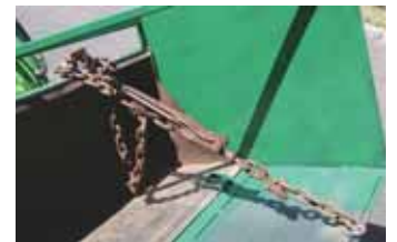
A pair of chain binders are attached to "tie-down" hooks welded onto bucket floor.
