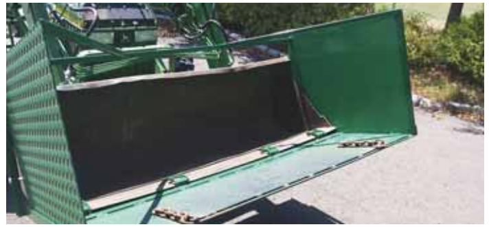
Bucket sides measure 30 in. high and floor extends 2 ft. in front of original bucket, with a 6-in. deep, 1/4-in. thick steel plate welded on front.
