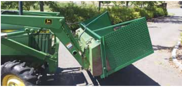
Kevin Daniels built this giant add-on bucket for his Deere 1070 35 hp, 4-WD tractor. It's built in one piece and attaches to loader's original 5-ft. bucket.
