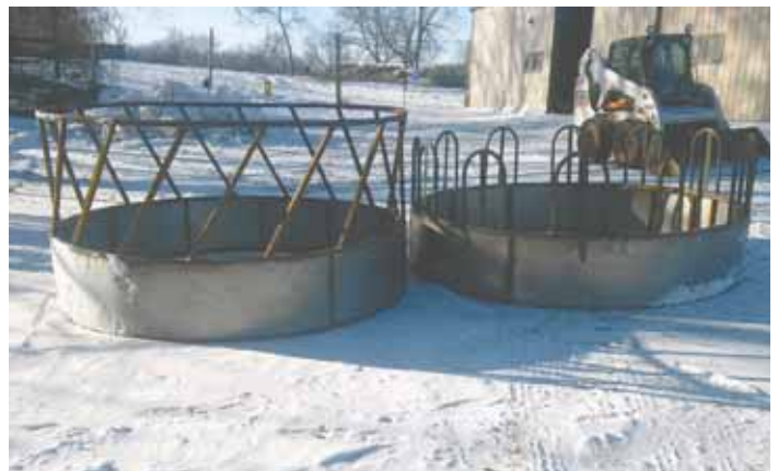
Each 8-ft. dia bale feeder is formed from steel rings and the spokes cut off reels.
