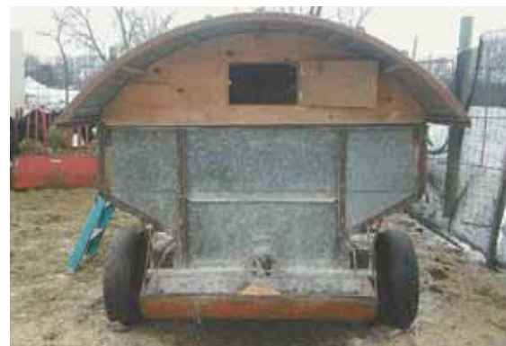
Jost also used the big reels to make a rounded steel roof over a feed wagon. Feeder tray on back was made from a scrapped auger tray.
