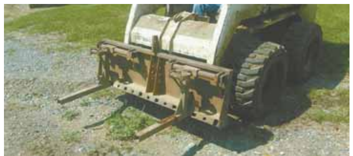
Dave Wampler converted a quick-attach, tined bucket on his Bobcat skid loader into this multi-use plate. He uses it to move forage harvester heads around, and for other hauling jobs.
