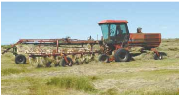
Dick Schirado turned a swather into a self-propelled rake by mounting the rake arms in place of the swather's header and mounting a dolly on the rake's drawbar.
