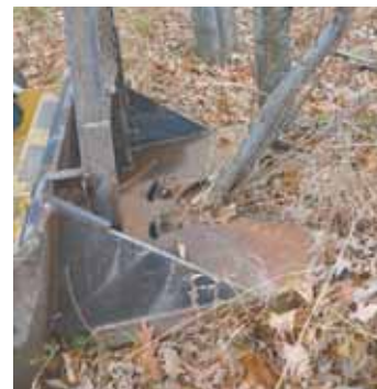
With the power of a 100 hp Deere track skid loader behind it, Tree Plucker plucks trees out roots and all (above). Spring-pressured jaws close and grab on impact, then open to release tree when skid loader stops.
