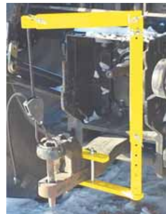
Spring-loaded pin puller yanks out the pin when tractor position is shifted.
