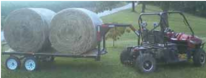
Chris Rahman uses the mini gooseneck trailer he built for his Polaris UTV to haul 2 big round bales at a time. Tandem axle trailer is 5 1/2 ft. wide and 10 ft. long with a stake bed.
