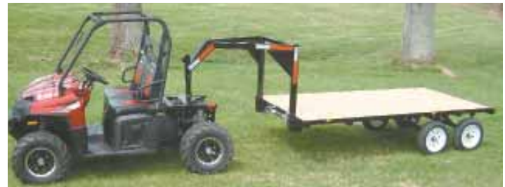
Chris Rahman uses the mini gooseneck trailer he built for his Polaris UTV to haul 2 big round bales at a time. Tandem axle trailer is 5 1/2 ft. wide and 10 ft. long with a stake bed.
