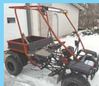
The new steering post came from an old lawn mower (left). He can add a cargo box on back when needed, as shown above.
