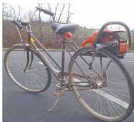
Jared Witmer attached a Husky chainsaw motor to the rear frame of his bike. “I start pedaling, and the compression starts the motor. When I hit the brakes, the motor stops,” he says.
