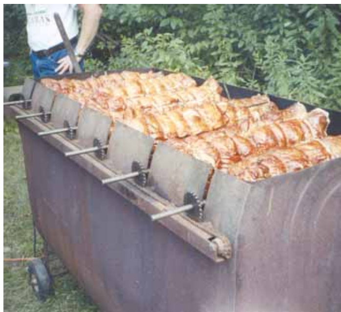
Roaster is fitted with six 3-ft. long “spits” which ride in 4-in. deep slots cut into both sides of tank. An electric motor drives a chain that rotates sprockets.
