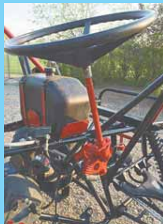
The new steering post came from an old lawn mower (left). He can add a cargo box on back when needed, as shown above.
