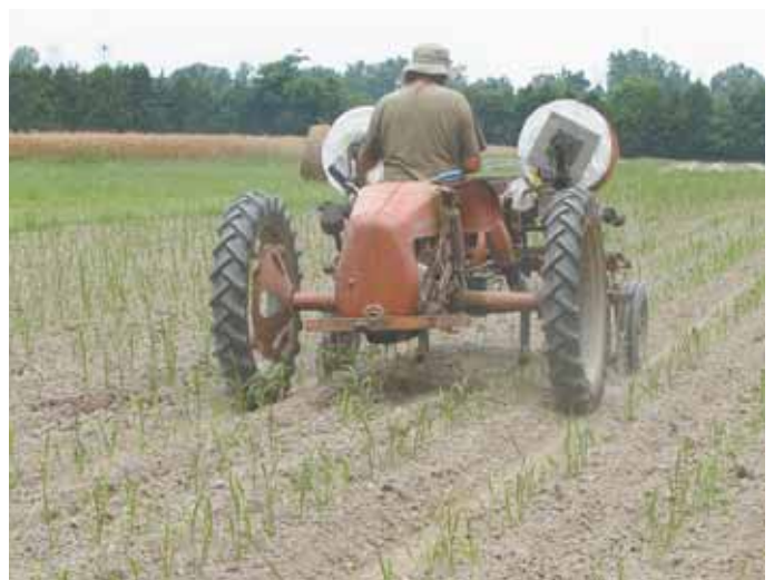
Thomet rigged up this tractor to lay drip tape along rows.
