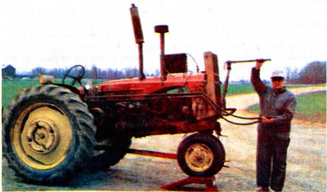
Willis Homer is shown holding the clutch and throttle lever in his right hand and the hydraulic hoses in his left.
