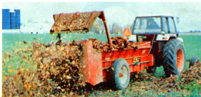
The biggest challenge faced was coming up with a way to spread leaves evenly across the field. A rear-unload manure spreader works best, researchers found.
