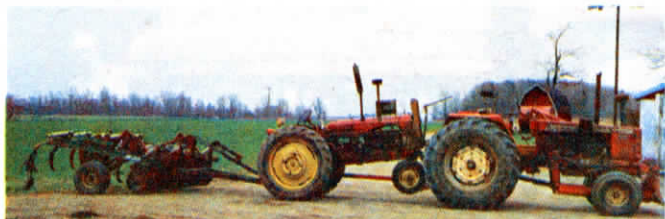
Homer uses the hooked-together tractors to pull a 14-ft. offset disk followed by a 9-shank Soil Saver.
