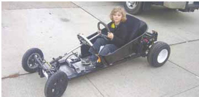
The driver rides in a wheelbarrow on this go-cart. Adjustable electronic speed controls limit how fast kids can go.
