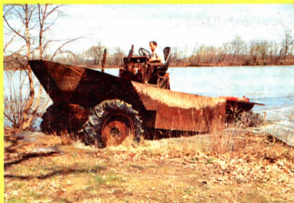
Home-built 30-ft. long tractor-boat can cruise down the road at 50 mph or navigate across deep water, propelled by the tractor tires.
