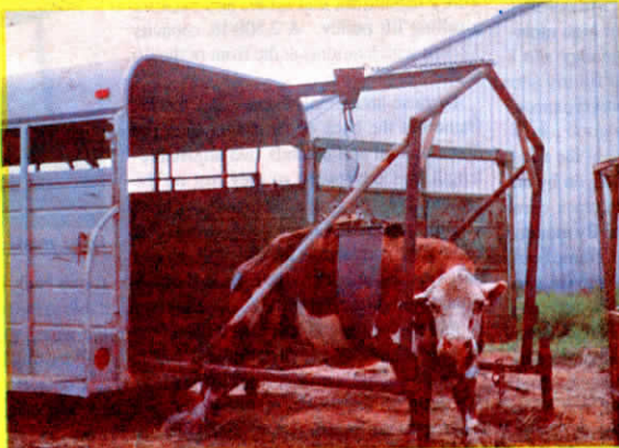
Rolling lift frame lifts cow and then rolls it into trailer for transport.
