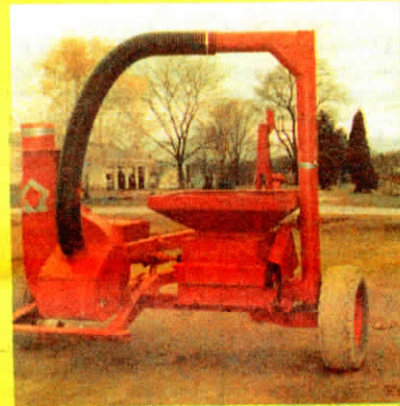
James Skelton, Edinboro, Penn., mounted a roller mill on the frame of a New Holland chopper to crack high moisture corn and blow it into his silo.
