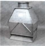
Our new "Spout Line Buster" is a grain distributor that attaches to the end of the spout on an unload auger to distribute foreign material and dockage throughout the grain in a load. As the flow of grain enters into the unit, it's split into two streams and passes over a series of specially designed screens and baffles that remove a portion of the foreign matter and then distributes it throughout the rest of the load.
