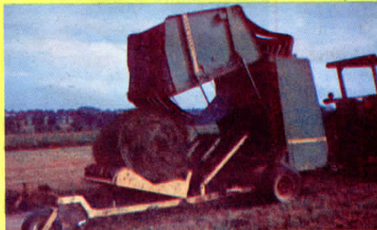
Baler discharges bale onto turntable (above). The machine then wraps it while the baler starts its next bale (top). Wrapped bale drops onto drag-behind canvas that prevents punctures in plastic.
