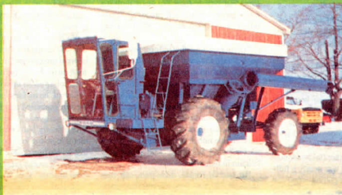
Old Combine Makes Great Self-Propelled “Grain Buggy”
