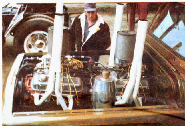
Two used 396 Chevrolet engines installed in the 1964 pickup are tied to transfer case salvaged from 2½ ton GMC military truck.
