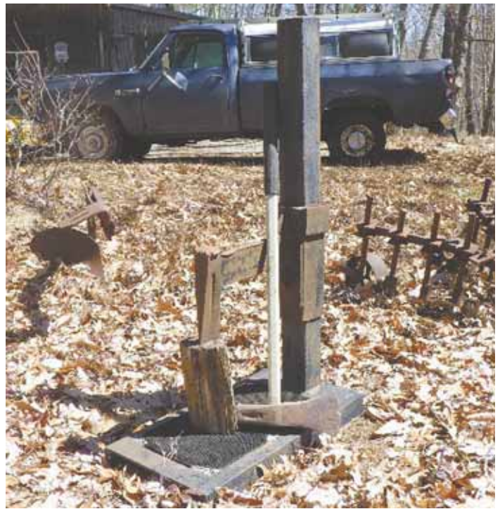
Splitting wedge is attached to an arm that slides up and down on a steel post. Wilcox lowers wedge over the chunk of wood, then hits it with a heavy sledge.
