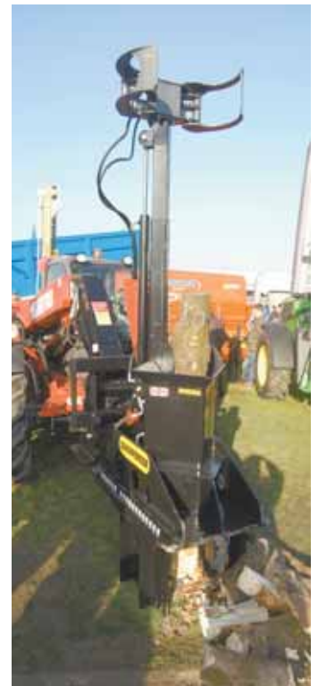
Loader-mounted processor picks up a log and rotates it vertically, then drops it into a cutting chamber equipped with a cutting and splitting shear.
