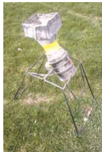
Garbage disposal is secured to metal stand and fitted with a hopper on top. Works great to mill shelled corn for chicken feed.
