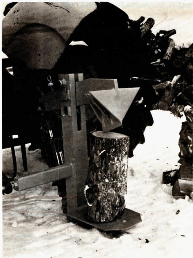
Forano splitter handles logs from 16 to 26 in. long. Mounts off to one side to clear the drawbar for towing wagons, trailers.
