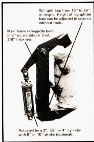
Forano splitter handles logs from 16 to 26 in. long. Mounts off to one side to clear the drawbar for towing wagons, trailers.
