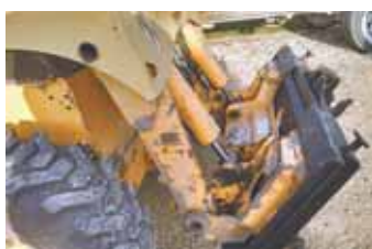
Brett Hundertmark made this low-cost quick-hitch for his Mustang skid loader by removing the 3-pt. quick-hitch brackets from his Deere tractor and welding them onto a new skid mounting plate.
