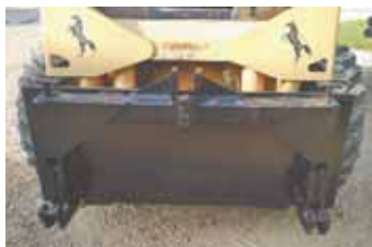
Brett Hundertmark made this low-cost quick-hitch for his Mustang skid loader by removing the 3-pt. quick-hitch brackets from his Deere tractor and welding them onto a new skid mounting plate.
