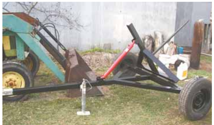
Two-wheeled mini mover can be used to move big round bales with a 20 hp Kubota tractor. Hinged spear is controlled by a hydraulic cylinder.
