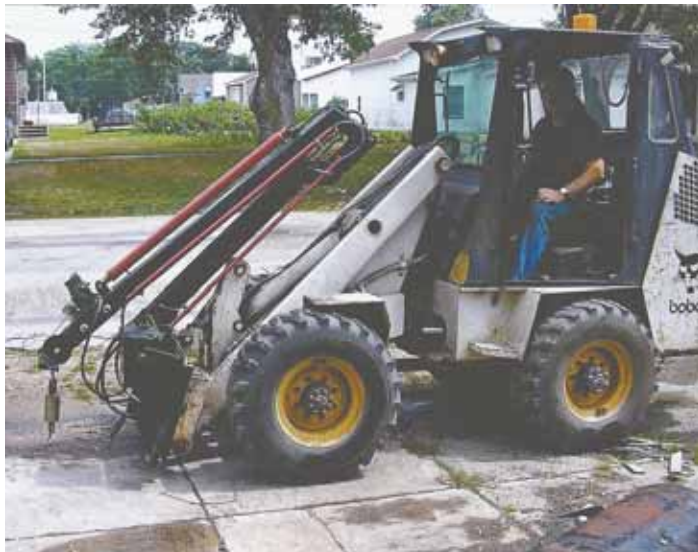
Compact "Cobra" crane is shown here attached to a Bobcat 1600 front-end loader but can also be attached to a skidsteer. Its 22-ft. boom folds up when not in use.
