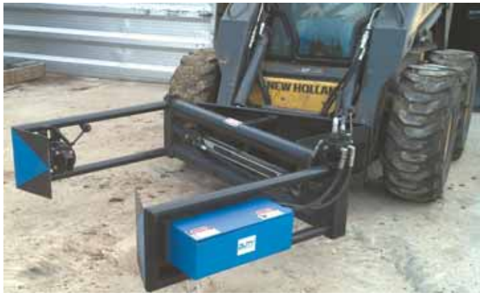
Skid loader-mounted attachment uses a spindle turned by a motor and gearbox housed in a box on side of attachment.
