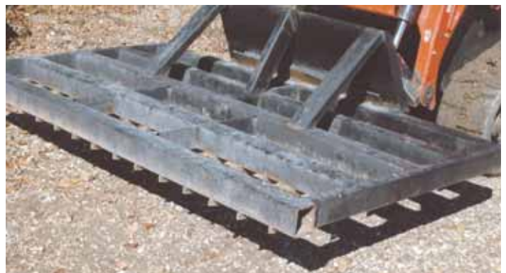
Perry Easley used the frame of an old chisel plow to build this 10-ft. wide pothole patcher, which he uses on his skid loader to smooth out gravel driveways.
