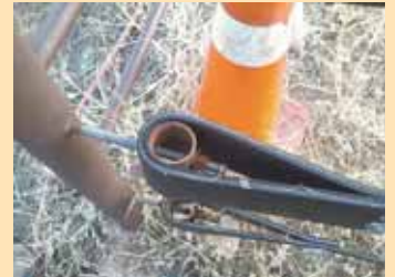
Belt is doubled over and bolted back on itself to form a loop. Pipe is then inserted inside loop and slid over rod. As belt stretches, operator tightens nut on rod to draw pipe and belt in.
