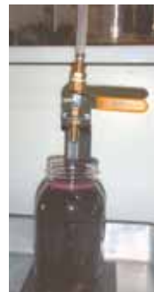
One end of transparent hose is attached to pressure cooker and other end to a fluid shut-off valve fastened to a metal stand. Turning the valve releases liquid into jar.
