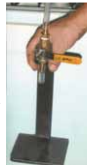
One end of transparent hose is attached to pressure cooker and other end to a fluid shut-off valve fastened to a metal stand. Turning the valve releases liquid into jar.
