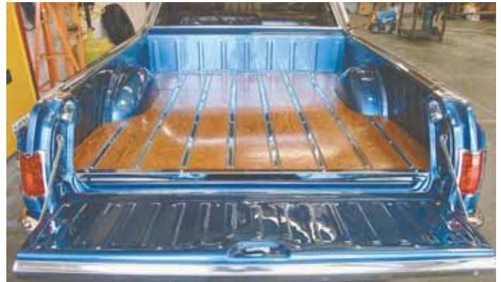
Wooden bed liner for pickups has a hardwood and stainless floor overlay. Bruce Horkey custom cuts the materials to fit all types of pickups.
