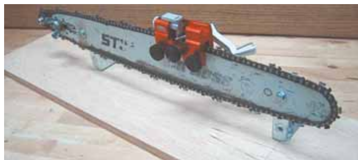
Bob Stewart likes his Timberline crank-type chainsaw sharpener. But instead of sharpening dull chains on his saw, he built a chain-holding stand from an old worn bar.
