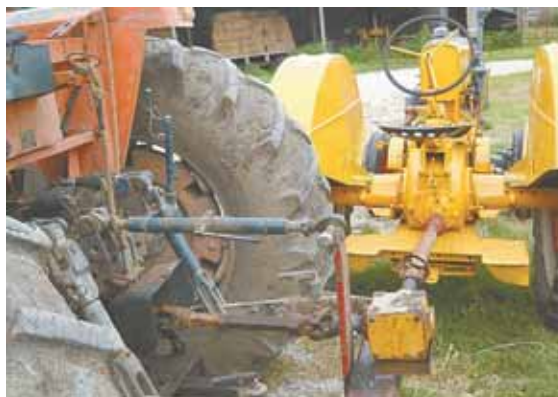
Maurice McCutchan uses an old grain auger gearbox to start old dead tractors. Gearbox is driven by his Kubota tractor's pto and hooks up to the dead tractor's pto.
