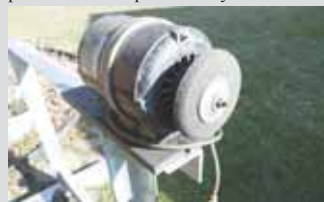
Bob Stewart likes his Timberline crank-type chainsaw sharpener. But instead of sharpening dull chains on his saw, he built a chain-holding stand from an old worn bar.
