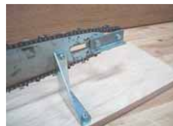
Bar mounts on a plywood base with 2 angle brackets. Homemade chain tensioner slides in bar slot.
