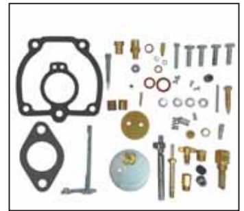
Steiner Tractor offers new carburetor kits for a wide variety of Farmall tractors. “Our kits have 90 percent of the internal components of a carburetor, so customers don’t have to piece their own kit together,” says Dan Steiner.
