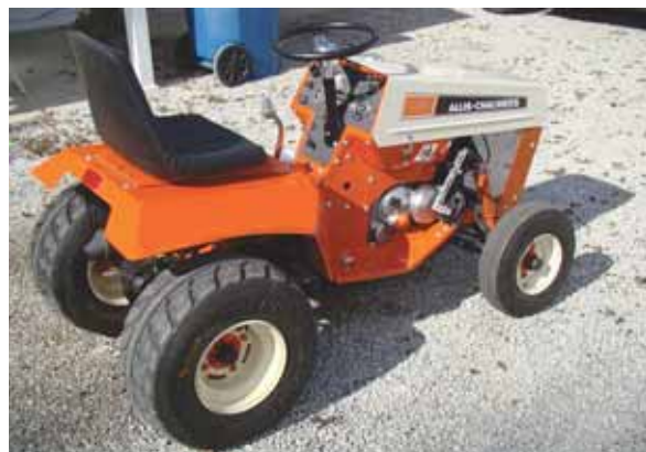
Mike Crutcher built this "ATV garden tractor" by combining a 1972 Allis Chalmers 410 garden tractor with a 1993 Kawasaki Bayou 220 ATV.
