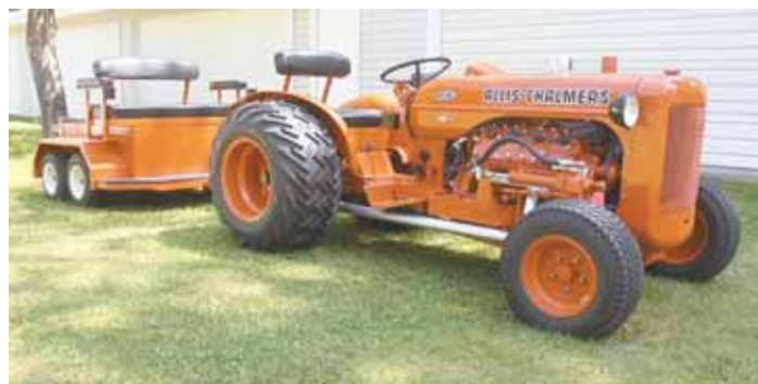
Mike Noonan's Allis Chalmers Mini B is only 36 in. tall, but it's powered by a 100 hp 1949 Ford flathead V-8 engine and has dual straight exhaust pipes that create a loud muscle car sound.
