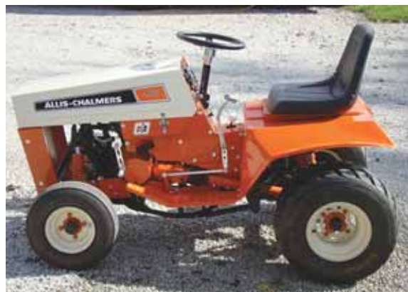
Tractor's 5-speed transmission is operated by a Hurst car shifter located on one side of operator platform. Shifter is connected by a long metal rod to transmission's shift linkage.
