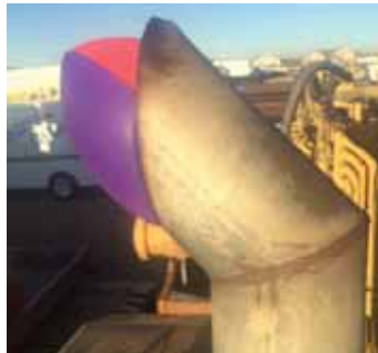
Photo at left shows a large Nerf football in a 5-in. dia. exhaust. Footballs can be cut in half, making them easier to compress to fit inside the exhaust pipe.
