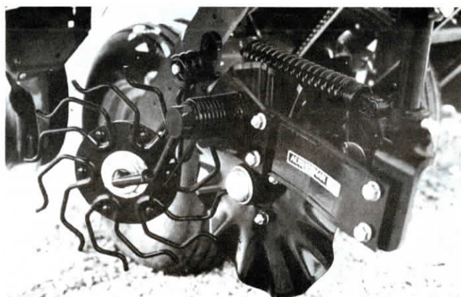
"Terra-Tine" row cleaner features a "foot" that limits tine depth and keeps trash from wrapping.
