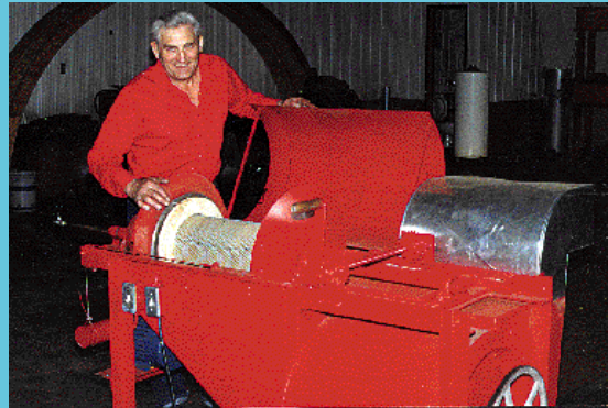
Stan Lapnisky's filter cleaner uses compressed air from inside the filter to blow dust out and a fan to vacuum it away.
