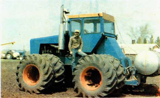
Larry Rauenhorst's "4-wheeler" was made from a 1965 Michigan wheeled dozer which he bought used for $4,000, including the engine.
