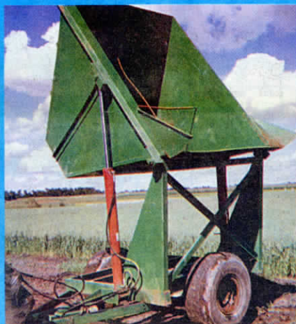
Home-built high lift 2-wheel dump cart allows Minnesota farmer Mark Spielman to load his fertilizer spreader right in the field. Story on page 2.
