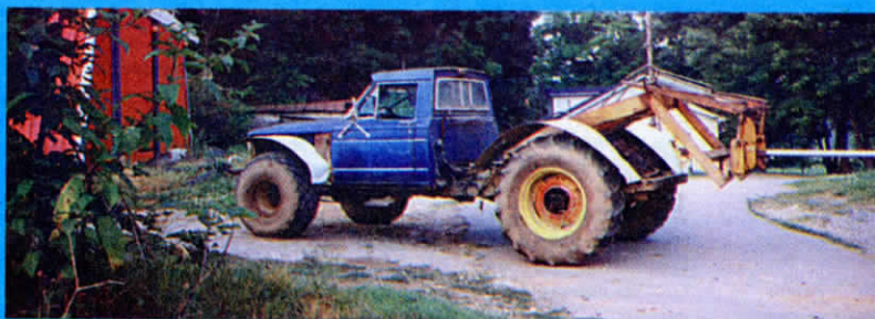
Delbert Cate converted a Jeep 4-WD pickup into a "Jeeptor" that's equipped with combine and tractor tires as well as a loader on back. He uses it to move 700 5 by 6-ft. bales a year. Story on page 2.
