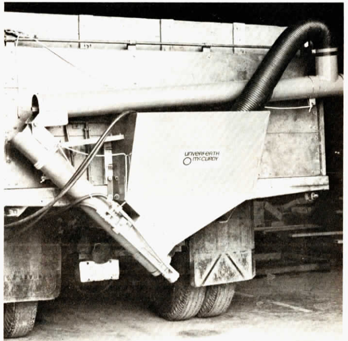
Auger and drive shaft hinge in middle and fold across tail gate for transport. Bottom cleanout allows auger to be by-passed when unloading grain or fertilizer out of truck box. Lists for $555.
